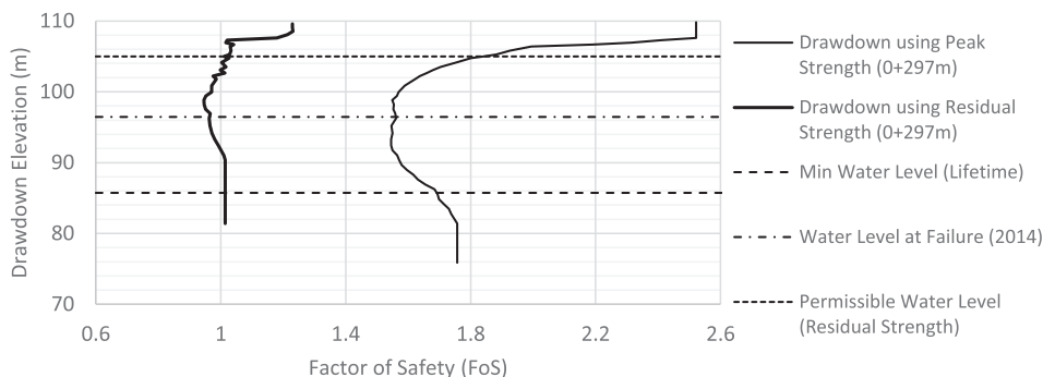
Fig. 15. Variation in the factor of safety with the drawdown level based on the peak and residual strengths.
